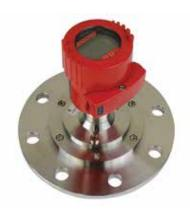
Non-contact radar continuously measures the level of powders, granules, solids, or liquids in a vessel. Reliable and precise in high dust, 80 GHz non-contact radar excels in powders and solids in tall and narrow vessels. Pulse radar transmitters using a lower frequency are more commonly used in liquids and perform in diverse tank shapes and environmental conditions.
