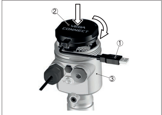
Fig. 36: Connection of the PC directly to the sensor via the interface adapter
