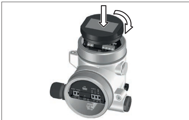
Fig. 33: Insertion of the display and adjustment module
