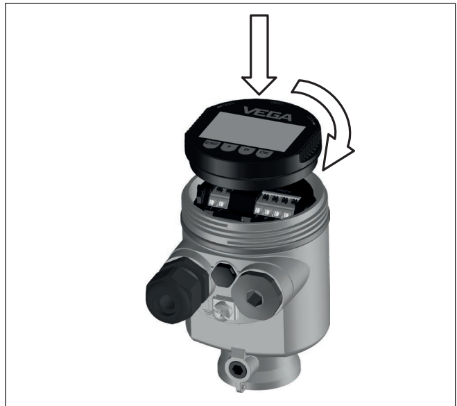
Fig. 41: Installing the display and adjustment module in the electronics compartment of the single chamber housing
