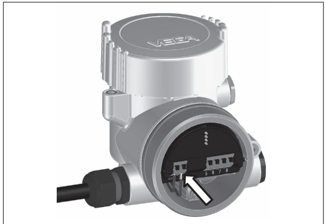
Fig. 27: Connection steps 5 and 6 - Double chamber housing
