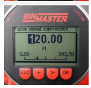
7. Screen should now show "Executing" with a processing bar underneath. When finished, "Change now" will show on the screen. Pres [ESC] key. False suppression for the actual distance to the product will be saved.
