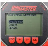
False signal suppression, use [>] and [+] keys to set the actual distance from the sensor to the product surface. Press [OK]
