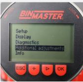
Additional adjustments, scroll to False signal suppression. Press [OK]
