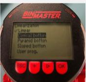
5. Set up the height of your cone. Press [OK]. Use the [esc] key to return to the main screen
