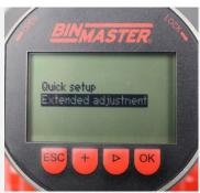
Scroll to Additional adjustments with the [>] key Press [OK]
