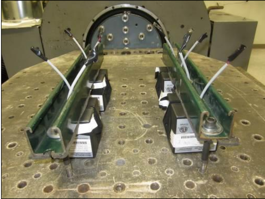
Photograph 5: Vibration Test Setup – Vertical Direction
