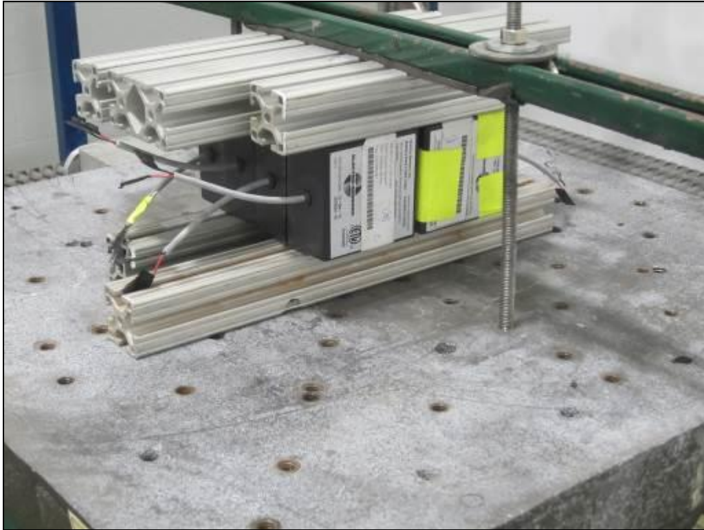
Photograph 8: Shock Test Setup – Lateral, Positive Direction
