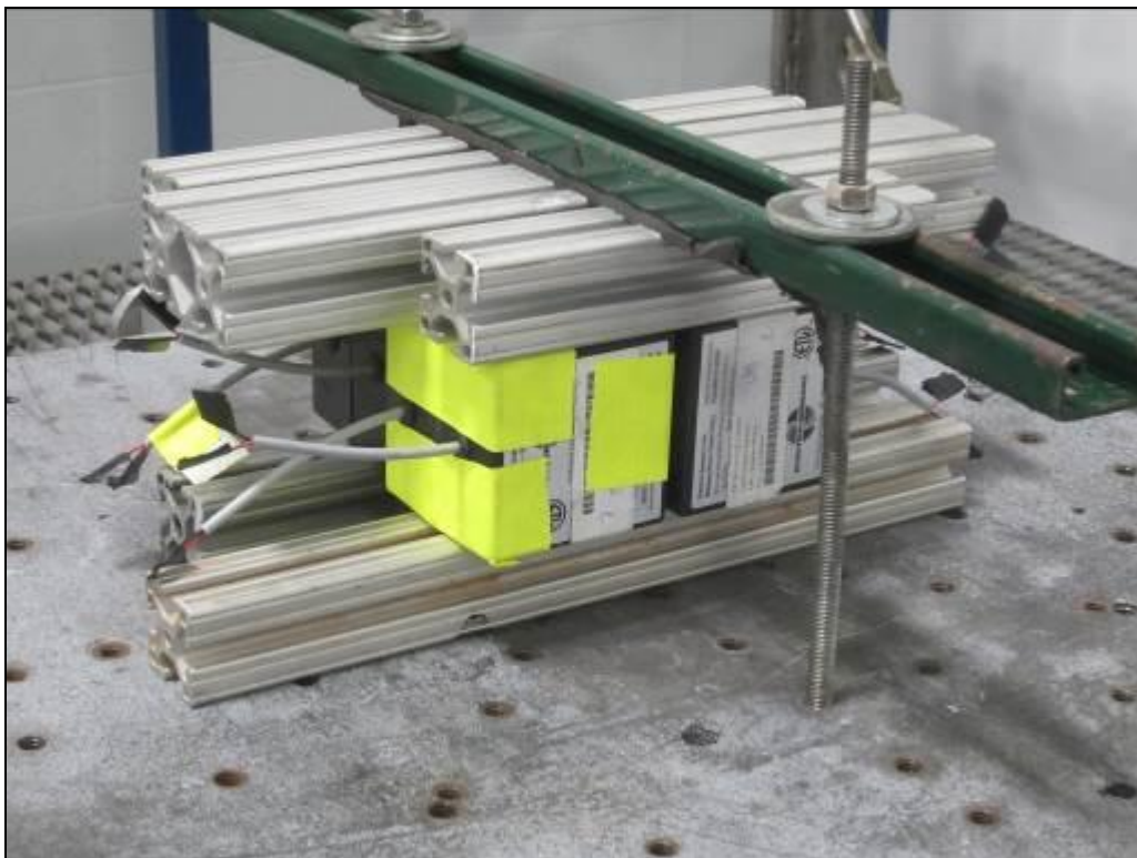
Photograph 9: Shock Test Setup – Lateral, Negative Direction
