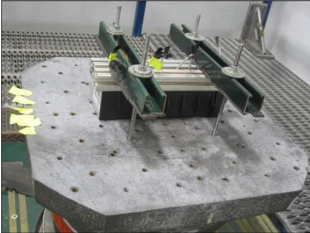
Photograph 6: Shock Test Setup – Fore/Aft, Positive Direction
