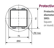
Protective tube length SRO with Tr 40x7-screw **Protective tube** w/o escape protection/ diameter anti-rotation device SRO: Incl. escape protection/ Square
